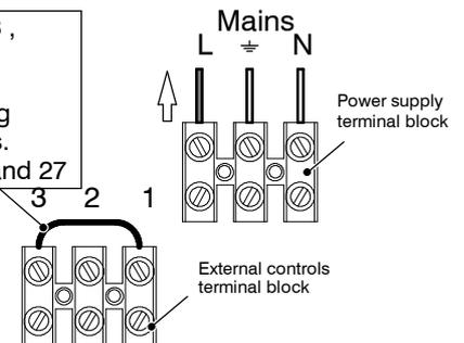
*Note: Ensure that the lengths of the current conductors are shorter than the earth conductor so that if the cable slips in its anchorage the current carrying conductors become taut before the earth conductor.*
