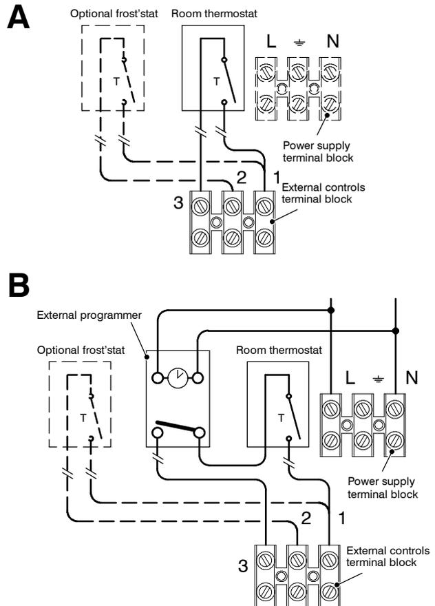
**N.B. These diagrams are schematic only and do not show external terminal strips etc.**
